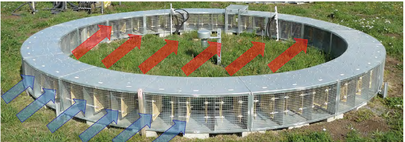
Giessen T-FACE - air Temperature warming and Free Air CO 2 Enrichment, with +2 °C air temperature and +20 % CO 2 , inside diameter: 4.3 m, start 2018; arrows = air flow in wind, blue = ambient temperature, red = +2 °C © Gerald Moser
