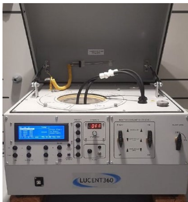
Abb. 9: Lucent 360 Advanced Photoreactor (Company: Hepatochem). © TU Darmstadt
