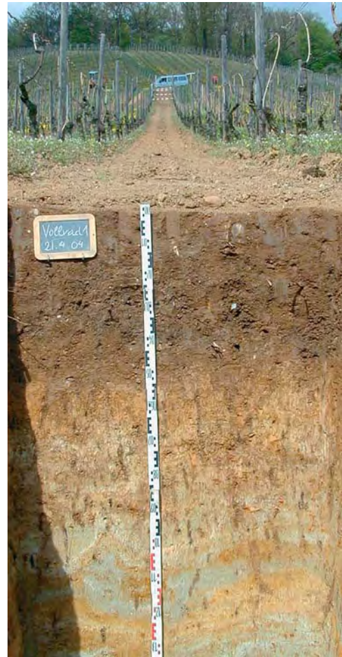
Fig. 2. Typical Rigosol with deep-ploughed modified topsoil to a depth of 55 cm over Tertiary marine sediments (Greifenberg).
